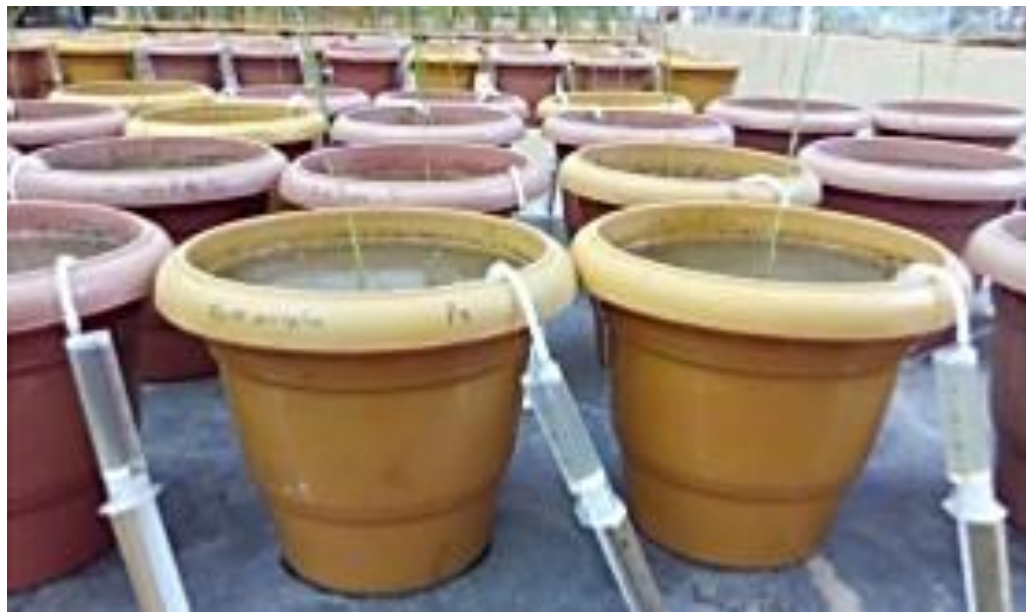
Plate 4: Overview of pots installed with rhizon samplers
