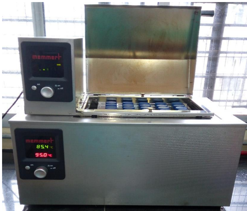
Plate 1: Hot water bath with horizontal shaker for extraction of organic Si pool
