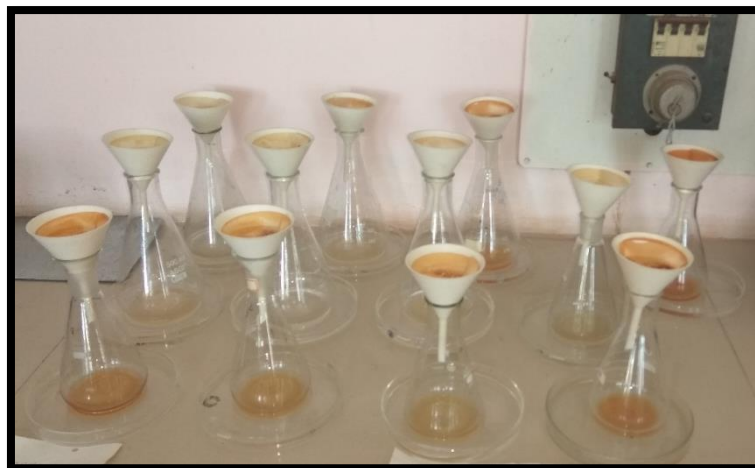
Plate 3.15 Determination of titratable acidity of banana powder
