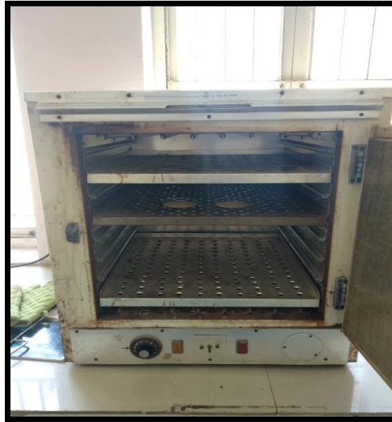
Plate 3.12 Determination of moisture content from banana powder
