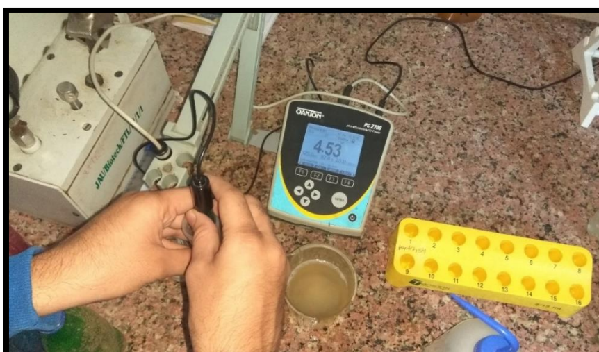
Plate 3.17 Determination of pH of banana powder
