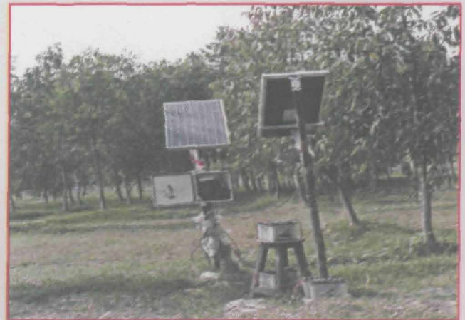
Figure 28. Measurement of transpiration rate with sap-flow meter
