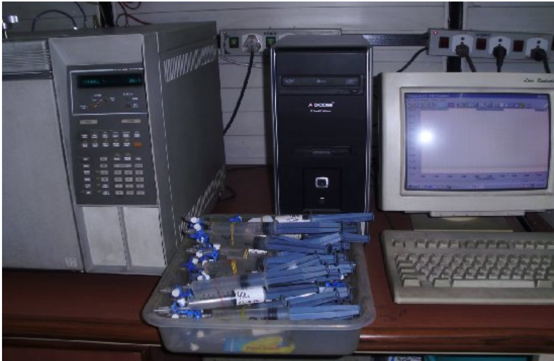
Figure 3.3: Gas chromatograph used for quantitative analysis of nitrous oxide emission
