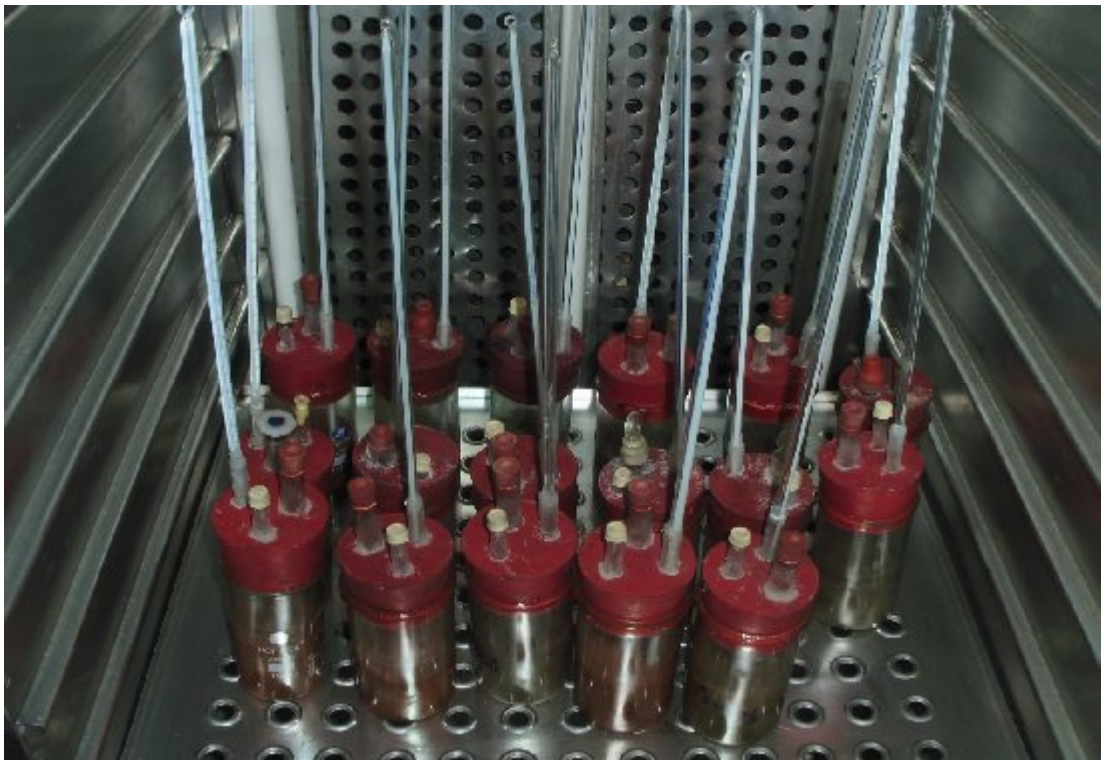
Figure 3.2: Experimental setup for measurement nitrous oxide emission from soil
