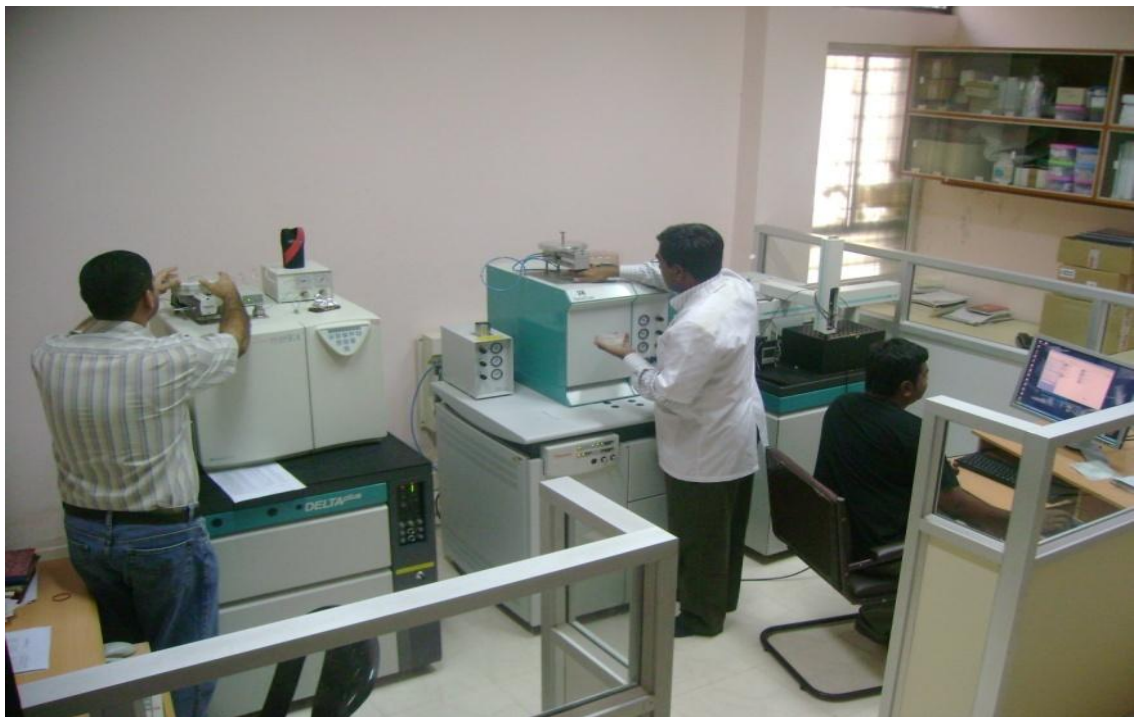
Plate 4: Isotopic Ratio Mass Spectrometer (IRMS) used for the determination of Carbon Isotope Discrimination
