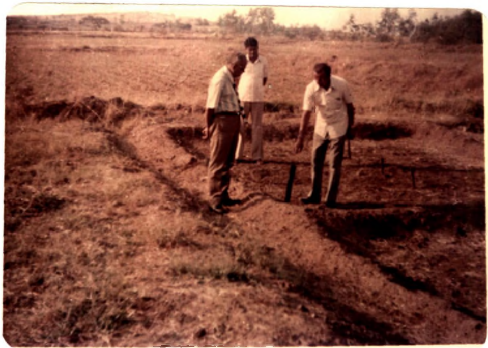
Plate 1. Explanation of the piezometer installation (observation wells) for water level recording
