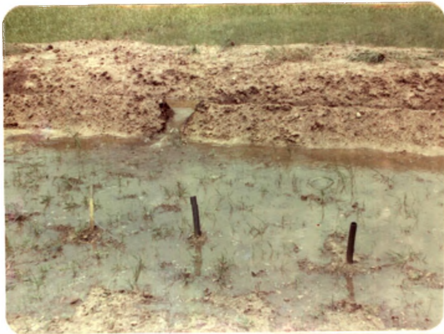
Plate 9. Picture showing the location of piezometers in each experimental plots.
