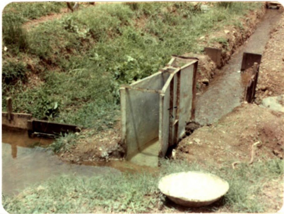
Plate 5. Use of Parashell-flume for measurement of irrigation water in experimentation
