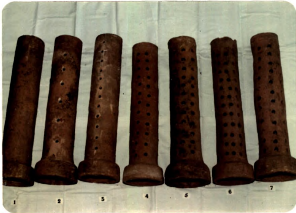
Plate 7. Tile with perforations of 0, 6, 12, 24, 36, 48 and 60 numbers per tile of 1 cm dia each.
