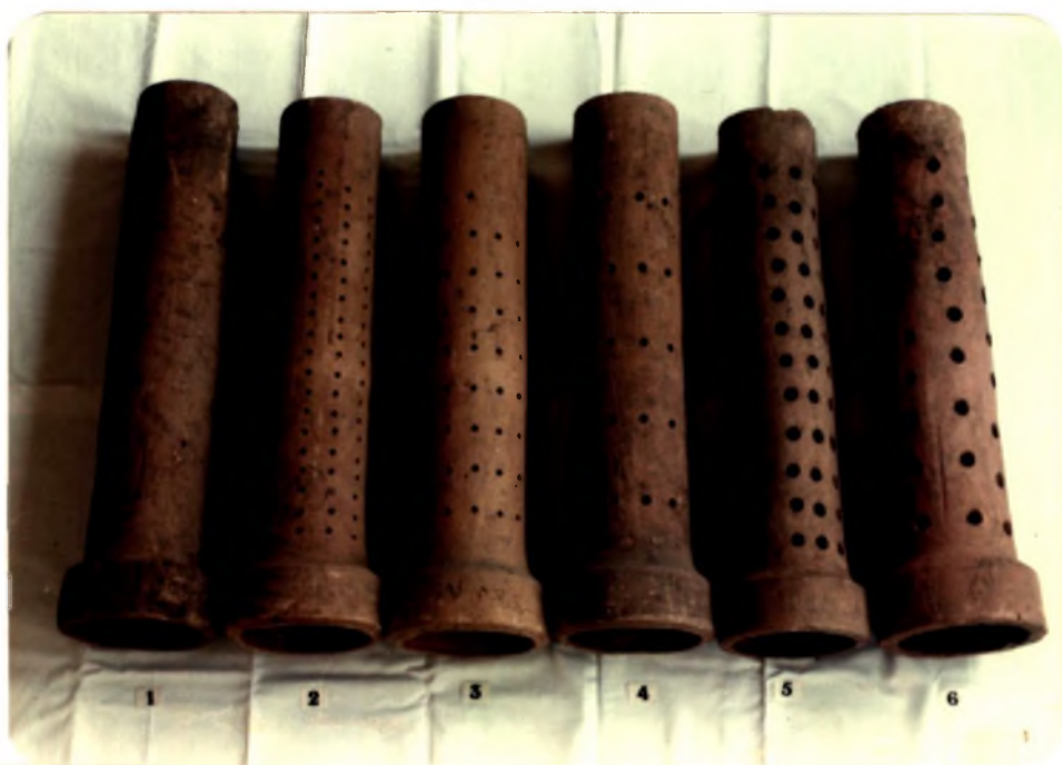
Plate 3. Tiles having perforations of 0, 0.50, 0.75, 1.00, 1.25, and 1.50 cm dia metre.
