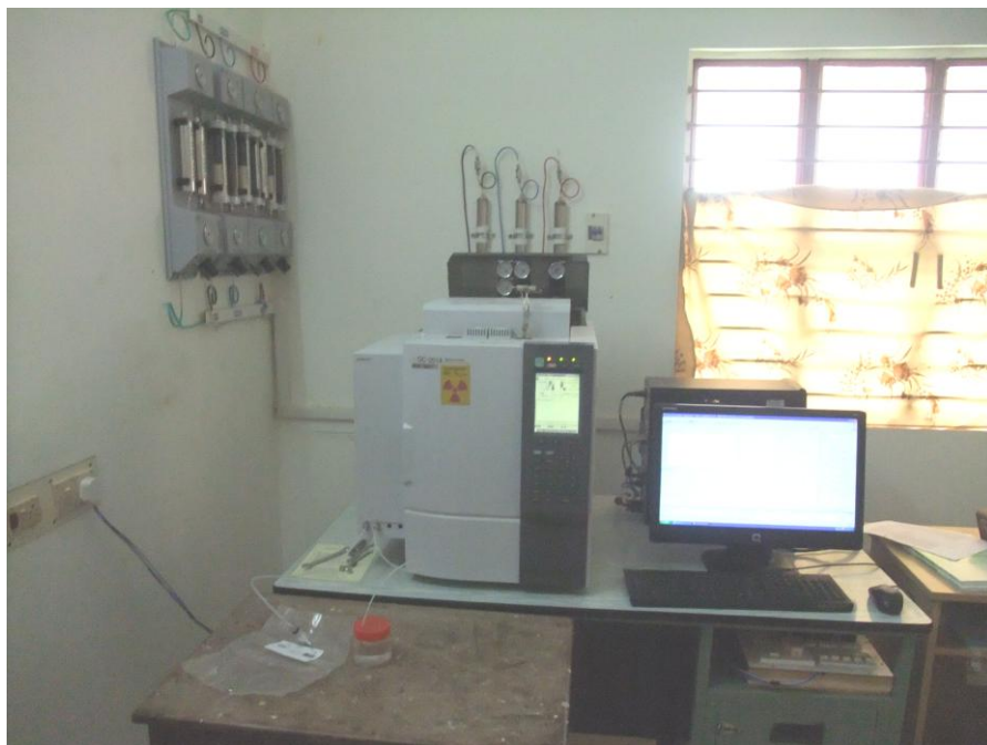
Plate 12. Methane analysis using gas chromatography
