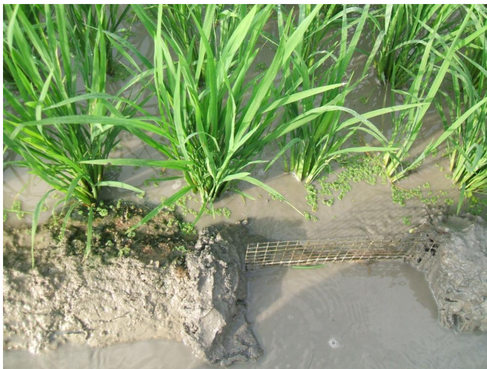
Plate 8. Collection of methane using methane collection chamber in the field
