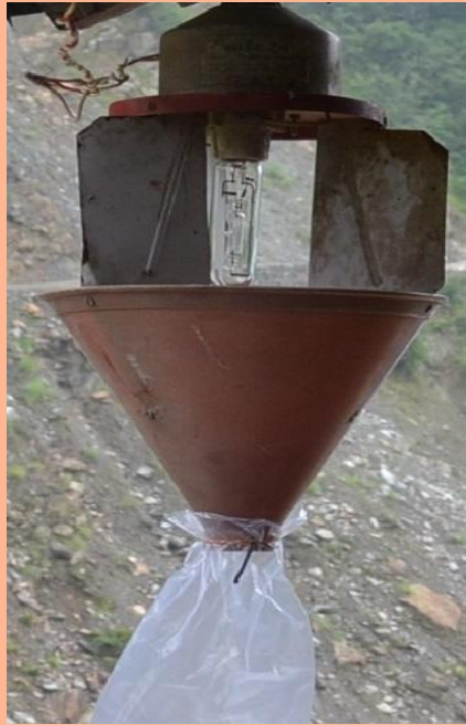
Plate 3.1 UV light trap used for monitoring of beetles
