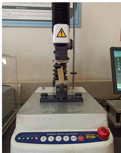
Fig. 3.18: Biodegradable cup sample placed in grip separator of texture analyzer for tensile force analysis
