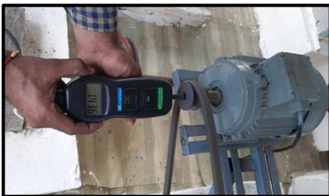
Plate 4.3 : Motor pully rpm of grader
