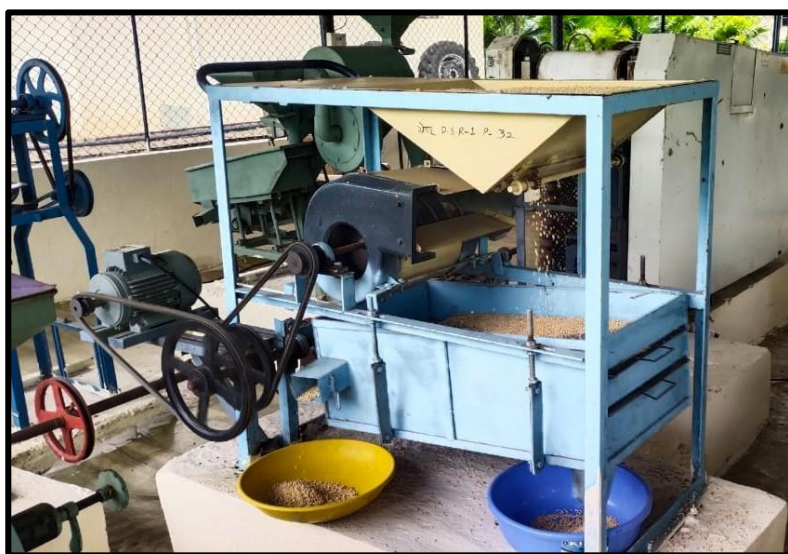
Plate 4.5 : Grain grader cum seed cleaner
