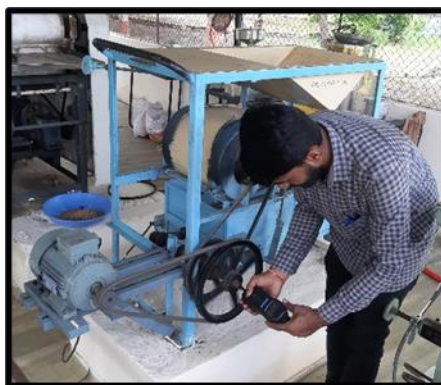
Plate 4.4 : Machine pully rpm of grader
