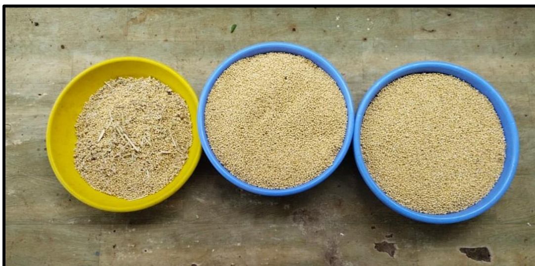
Plate 4.6 : Three grade of sorghum obtained from the solar powered grader cum cleaner
