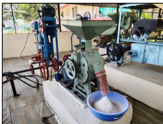
Plate 4.10 : Solar operated flour machine
