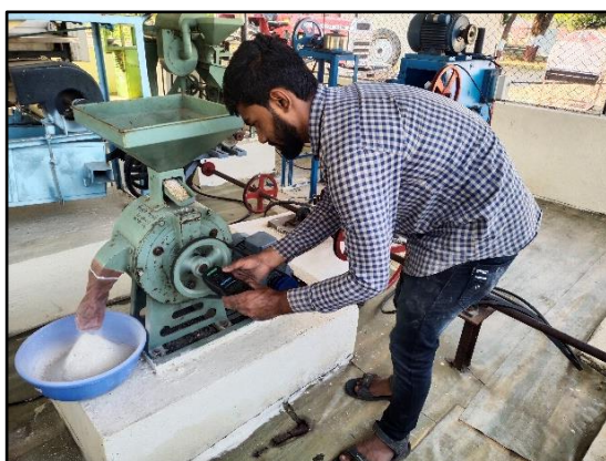
Plate 4.9 : Rpm measuring of flour mill motor
