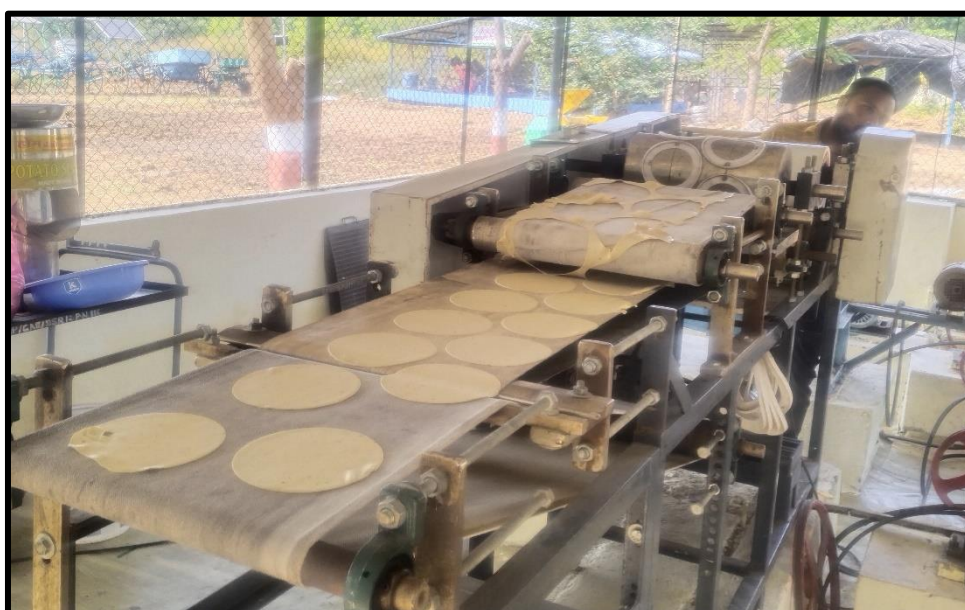
Plate 4.1 : Performance evaluation papad making machine
