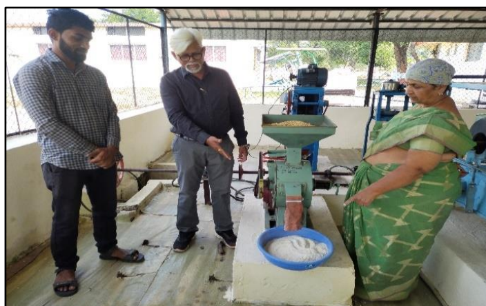
Plate 4.11 : Flour mill under operation using solar power
