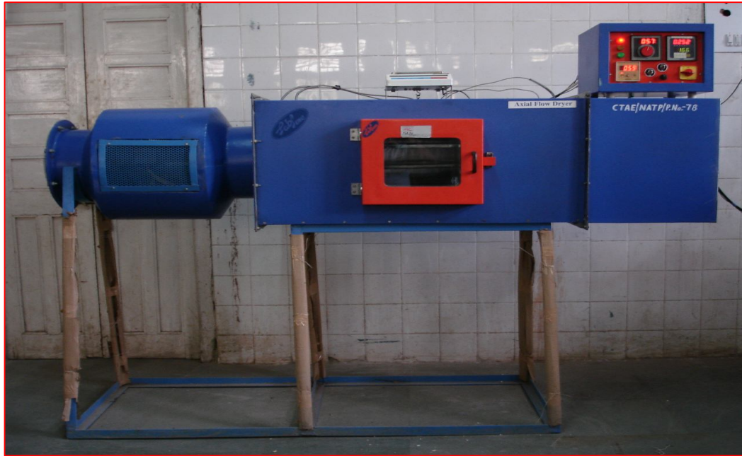
Plate 3.3 Experimental convective tray dryer
