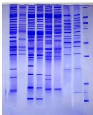
Protein profile in different salt hyperaccumulator plants under salinity (S2 = 16dS/m) and control (S0) through SDS - PAGE .
