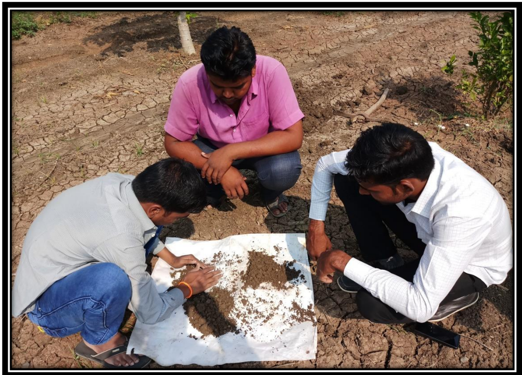
Plate no. 2 : Reduction of sample size by quartering method
