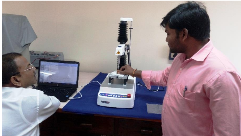
Plate 3.3: Experimental setup for determination of hardness of solid jaggery by using texture analyser
