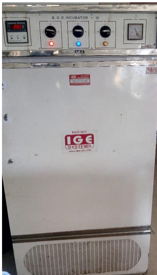
Plate 3.4: Experimental setup for determination of equilibrium moisture content of solid jaggery at temperatures of 25°C, 35°C and 45°C
