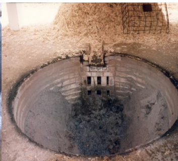
Plate 2.5: Traditional furnace for sugarcane jaggery
