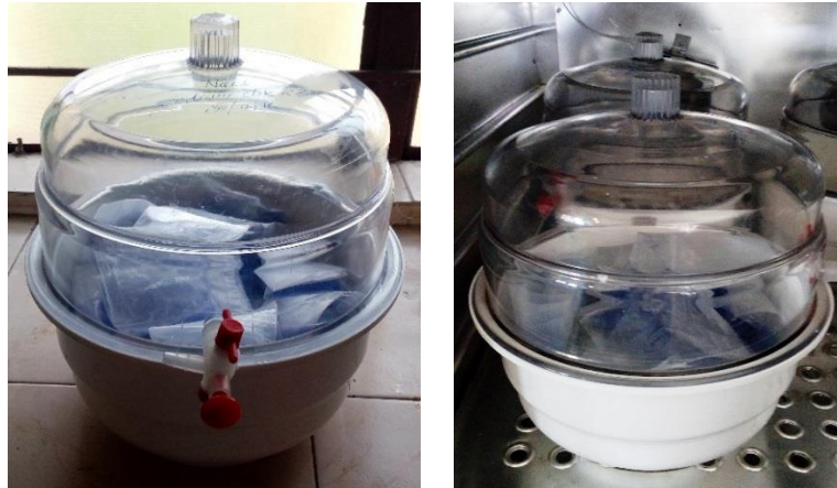
Plate 3.6. Experimental setup for determination of water vapour permeability for packaging material
