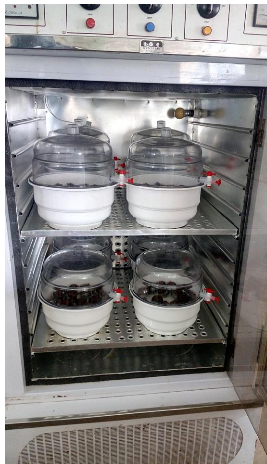
Plate 3.5: Incubator used for solid jaggery samples in desiccators at different controlled equilibrium relative humidities and at different setup temperatures
