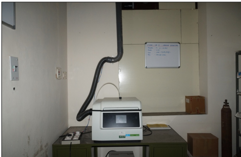
Plate 3A. Titan MPS Microwave Sample Preparation System
