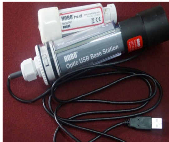
Plate 2B. HOBO Temperature humidity data logger with its base station and cable for down loading
