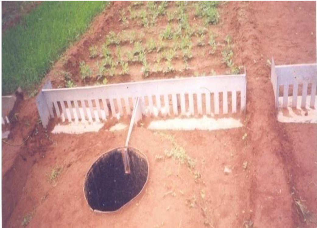
Fig 4.5 Multi slot divisor with runoff collection tank
