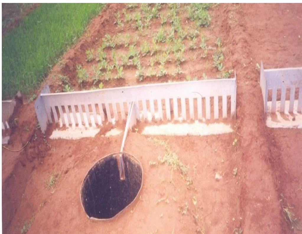
Fig.3.3 Multislot divisor with runoff collection tank
