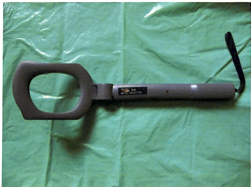
Fig. 12: Metal detector used in the study.
