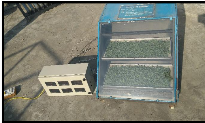
Plate 3.6 Drying of fenugreek leaves in solar cabinet drying
