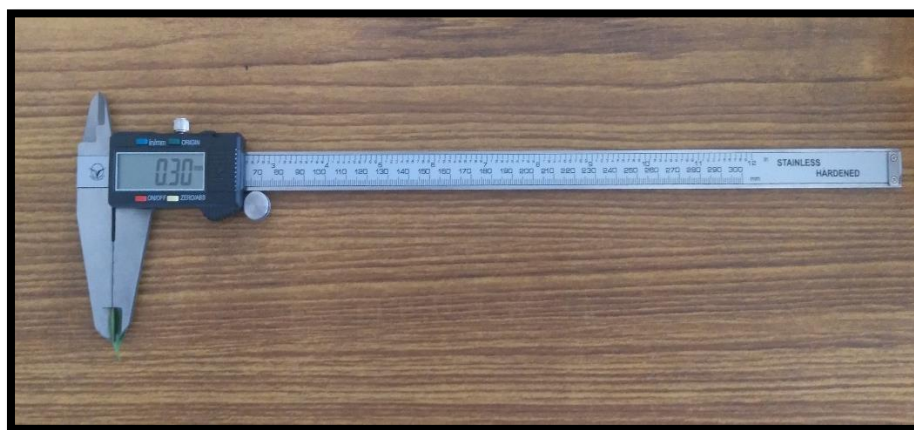
Plate 3.2 Thickness measurement of fenugreek leaves
