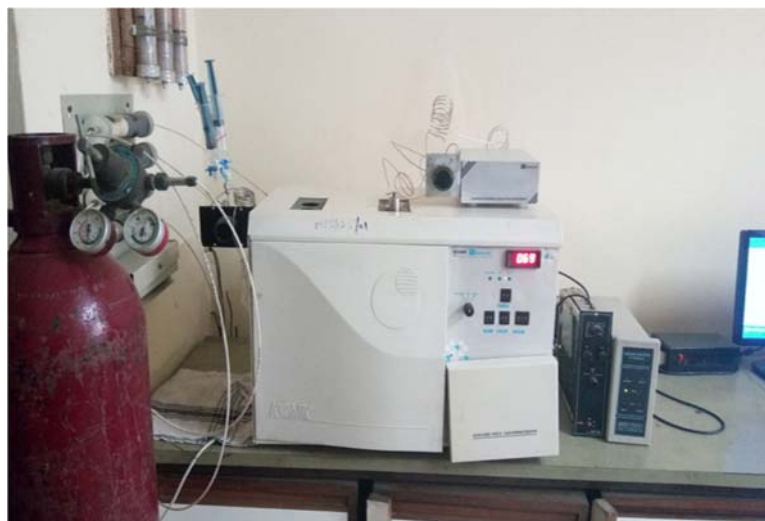
Plate 3.4: Measurement of GHG flux by Gas Chromatography
