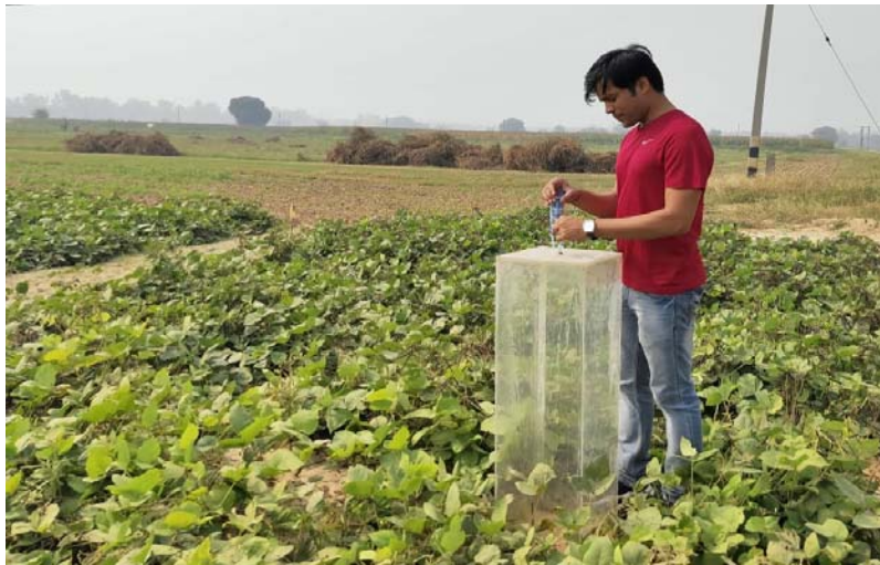
Plate 3.3d: Gas collection by closed chamber technique in mungbean
