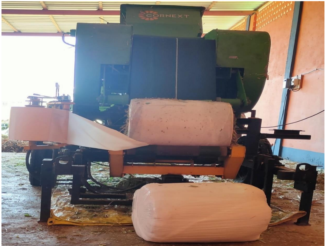
Fig 6. Silage bales making by using Silage bale making Machine MSB(500)
