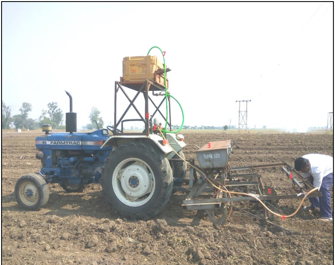
Fig. 3.8 Tractor operated seed ferti drill-cum-weedicide applicator
