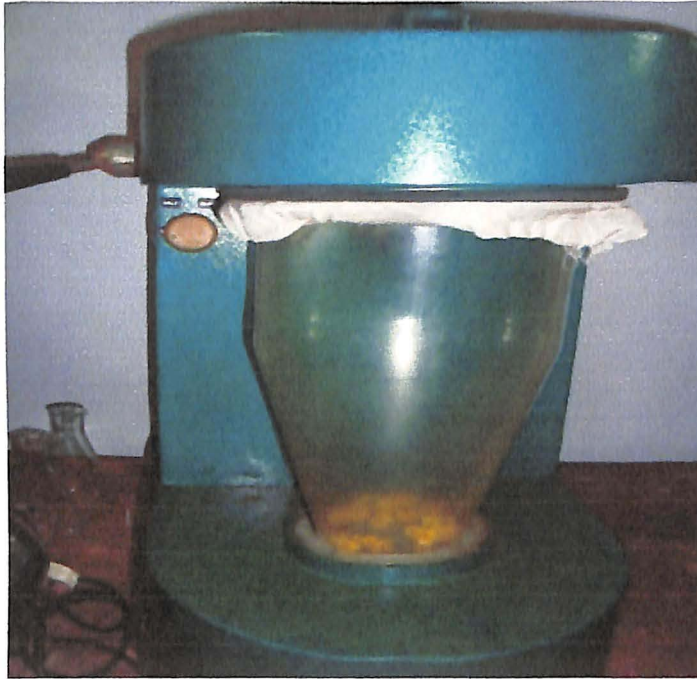
Plate. 3.5 Fluidized bed dryer used for drying of cornflake
