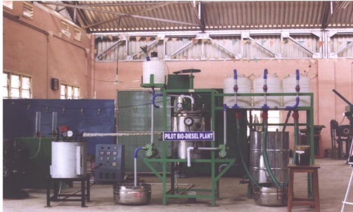
Plate 4.8. Biodiesel pilot plant
