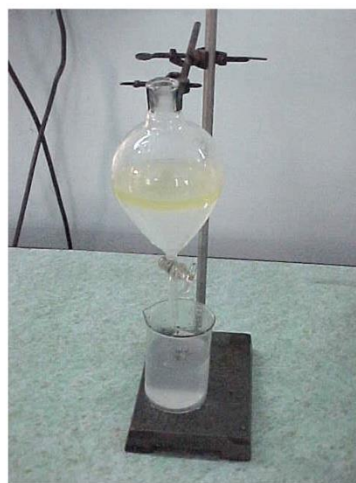
Plate 4.2. Biodiesel washing in separating funnel
