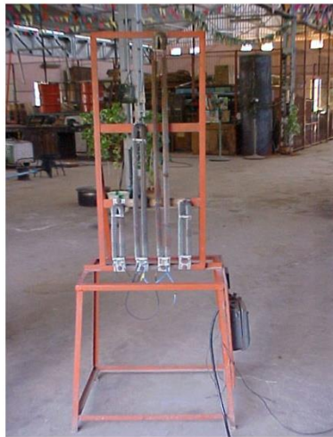
Plate 4.11. Electrical loading unit
