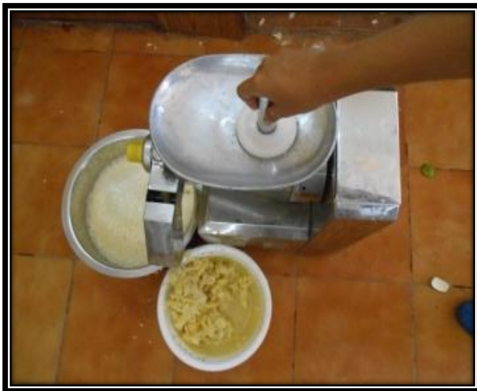
Plate 2. Power operated screw press type juice extractor
