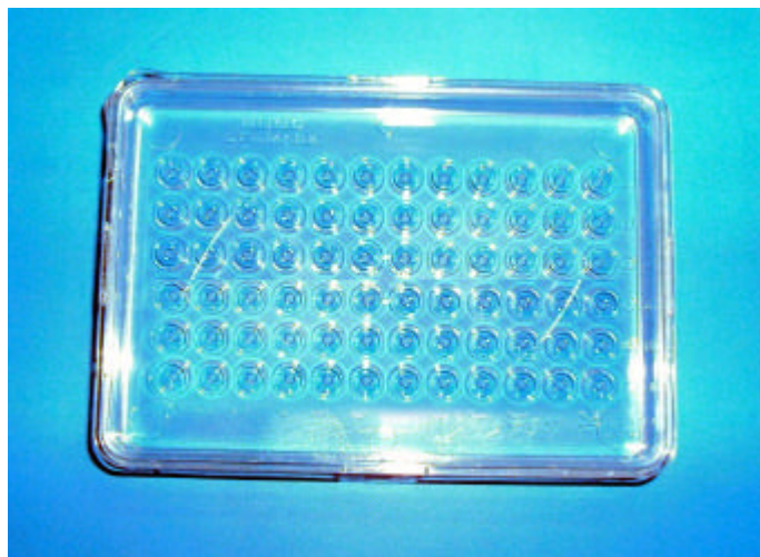
Fig.2b: Terasaki plate used for titration of rabies virus by fluorescent antibody technique.
