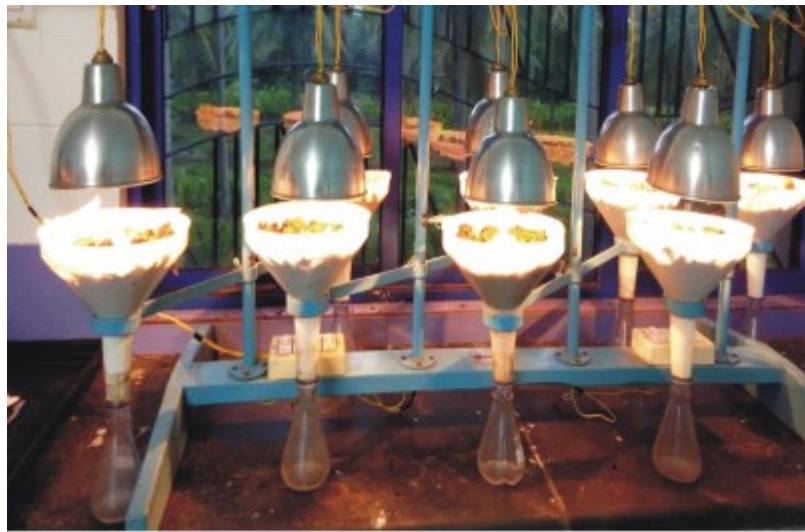
Berlese funnel setup for extraction of meso arthropods
