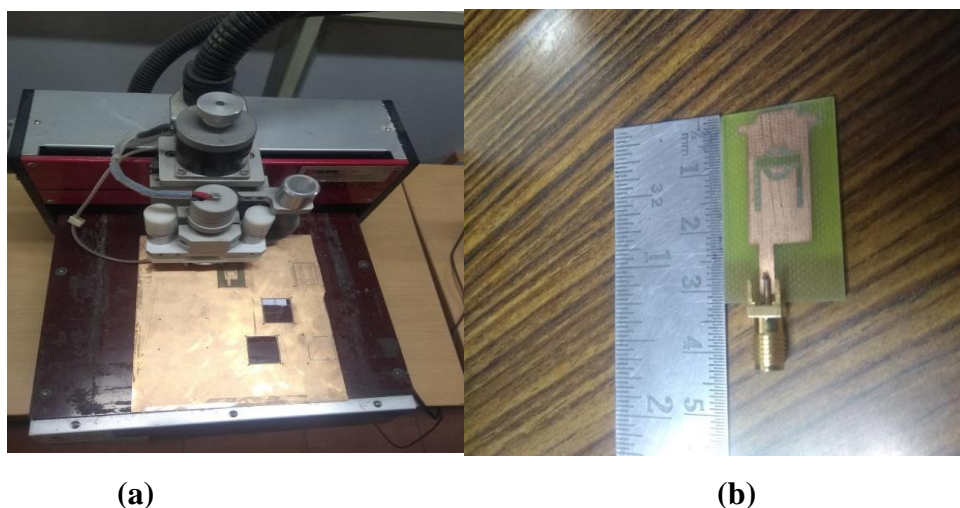
Fig. 3.24: (a) PCB prototype machine (b) Fabricated proposed antenna
