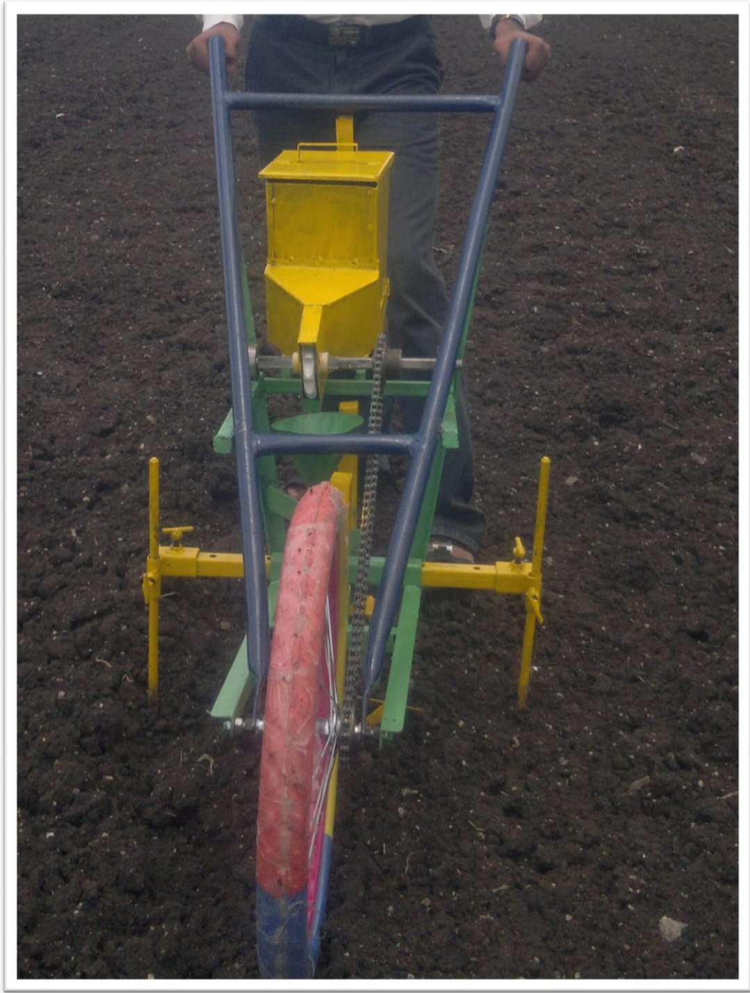
Plate 3.1 Front view of manually operated single row multicrop planter
