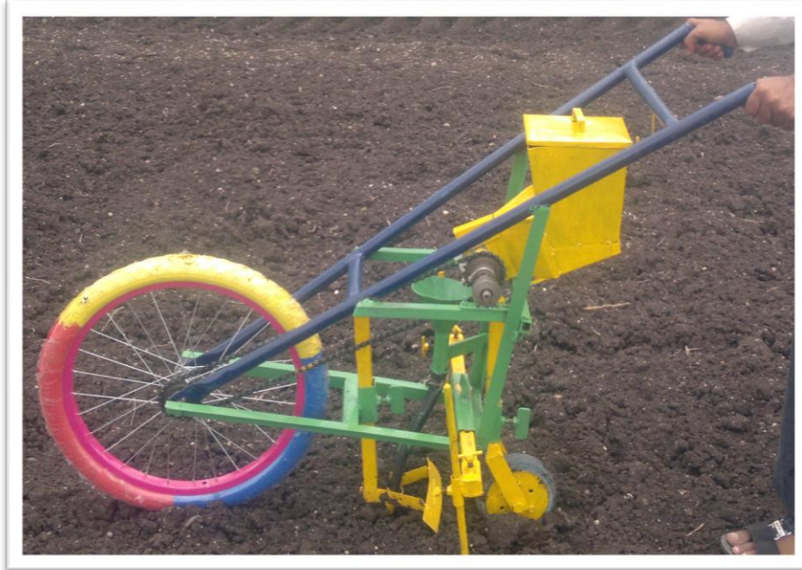
Plate 3.2 Side view of manually operated single row multicrop planter
