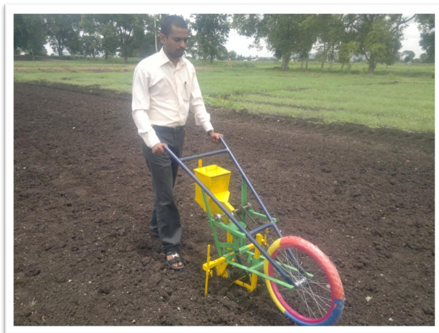
Plate 4.2 Manually operated single row multicrop planter in operation
