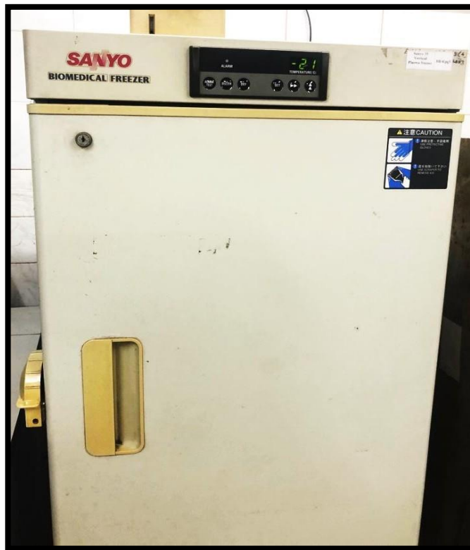
Plate 3.8 Biomedical Refrigerator for storage of Plasma at -20 0 C
