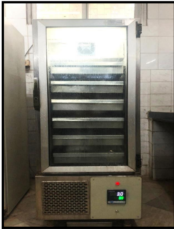
Plate 3.7 Blood Bank Refrigerator for storage of Whole blood at 4 0 C
