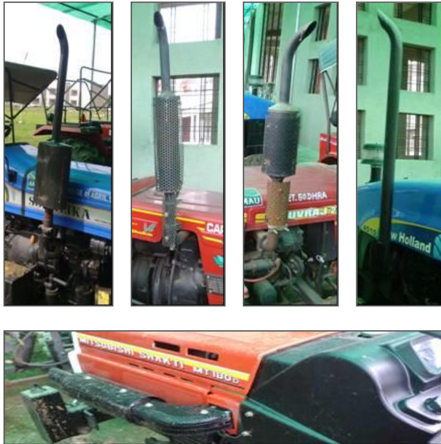
Fig. 1.1: Different exhaust silencers used in different makes of tractors
