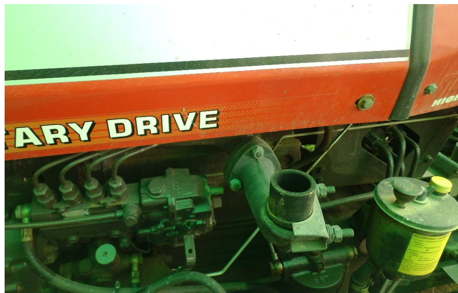
Fig. 3.23: Exhaust outlet of Tractor-2
