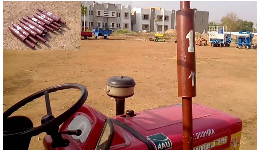
Fig. 3.26: Noise SPL testing of Tractor-1 (Mini Tractor) under different mufflers
