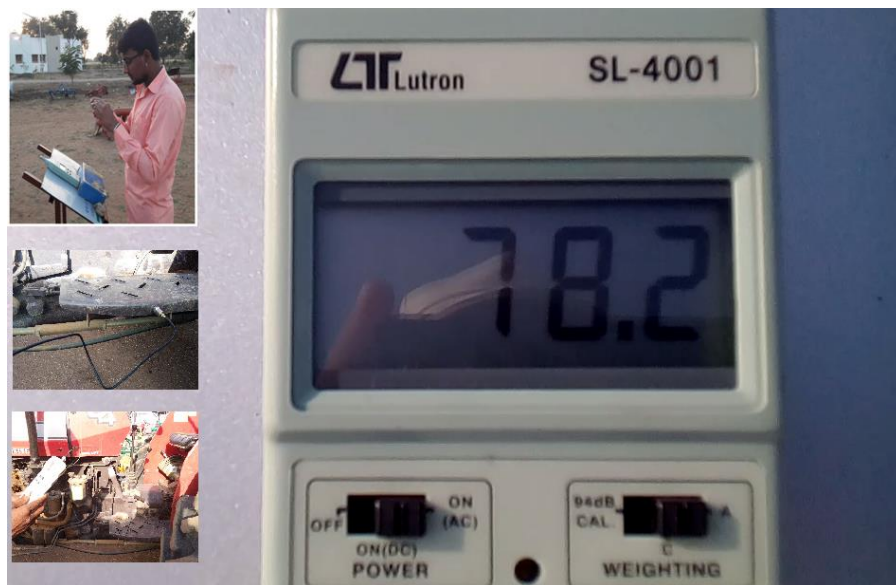
Fig. 3.27: SPL (Sound Pressure Level) observation being recorded on sound level meter (SL-4001) and vibration measuring on footrest
