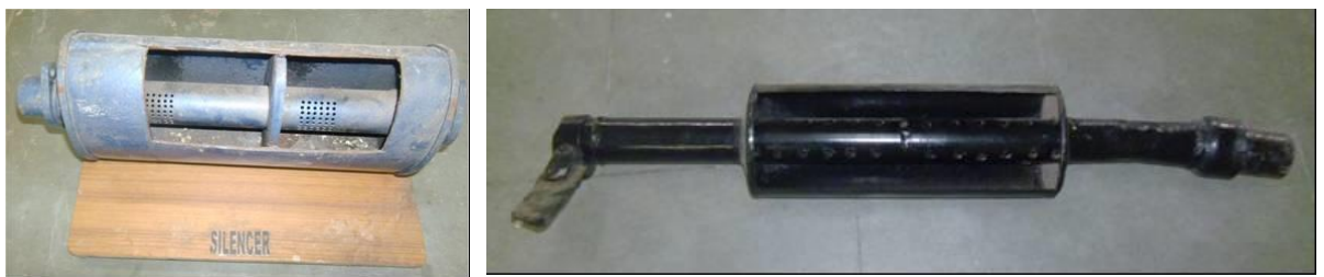
Fig. 3.10: Cut section models of exhaust mufflers at FMPE lab of CAET, AAU, Godhra.
