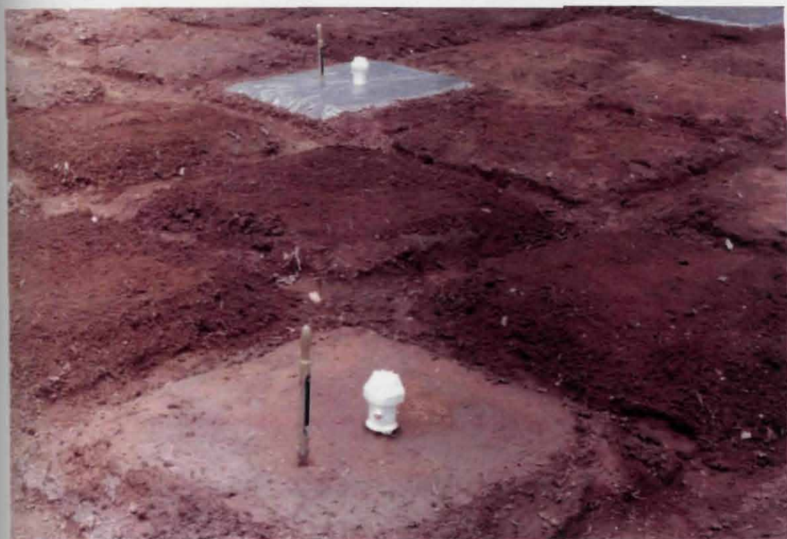
Plate.26: Photograph showing soil thermometers for measurement of temperature.
