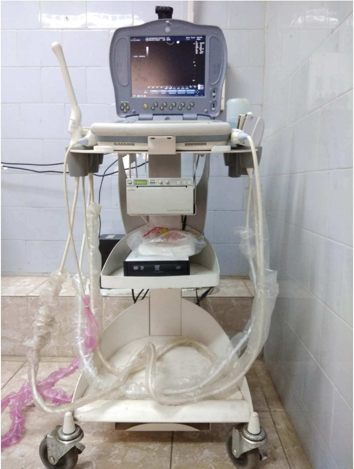
Plate 03: Logiq Book XP from General Electronics with microconvex transducer of 6 to 10 MHz capacity
