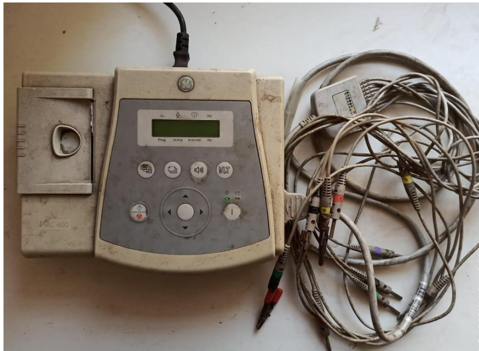
Plate 02: GE's MAC 400 (Wipro GE Health care Pvt. Ltd, Bengaluru) 3 channel, 12 lead electrocardiograph
