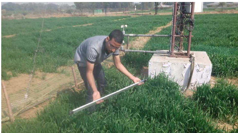
Plate 5. Measurement of PAR using line quantum sensor during rabi , 2017-18
