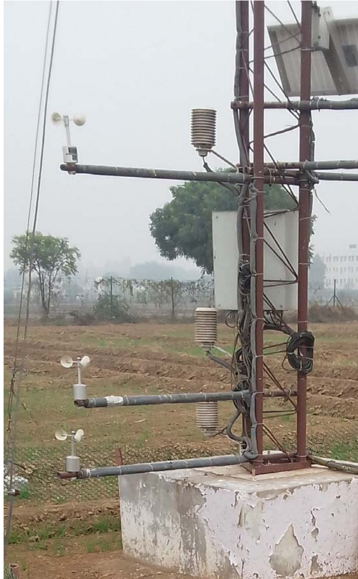
Plate 2. Micrometeorological tower with temperature, humidity, and wind speed sensor at various height (0.5m, 1m, 2 m)
