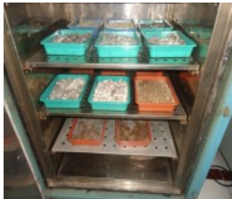
Scale up studies using tray fermentors
