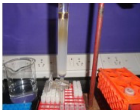
Gel filtration chromatography using Sephadex G100
