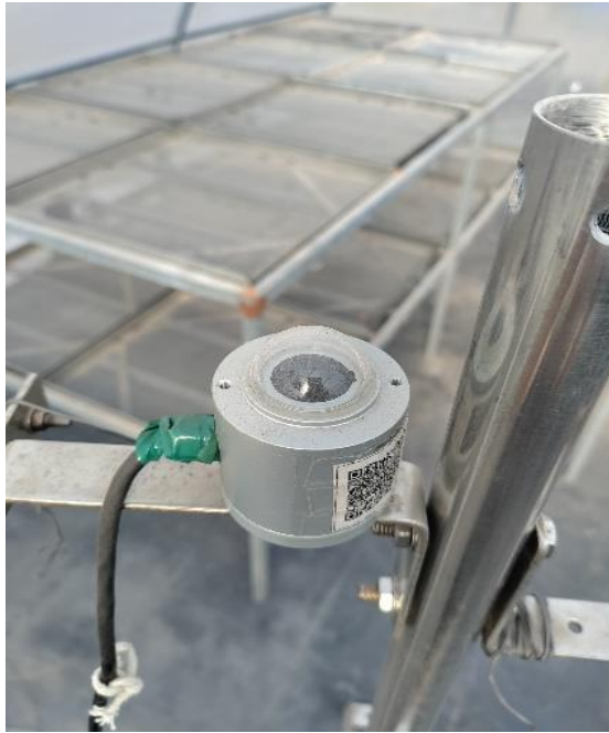
Plate 3.9 Pyranometer for measurement of global solar radiation
