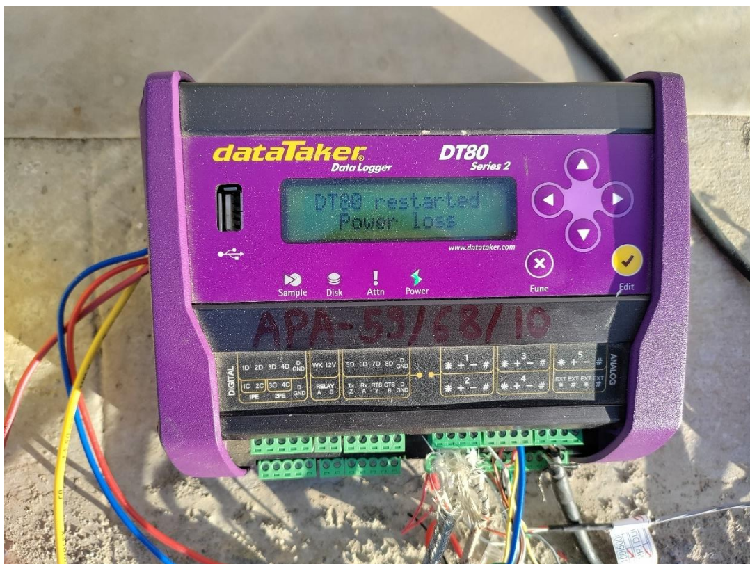
Plate 3.10 Data logger to record the microclimate data
