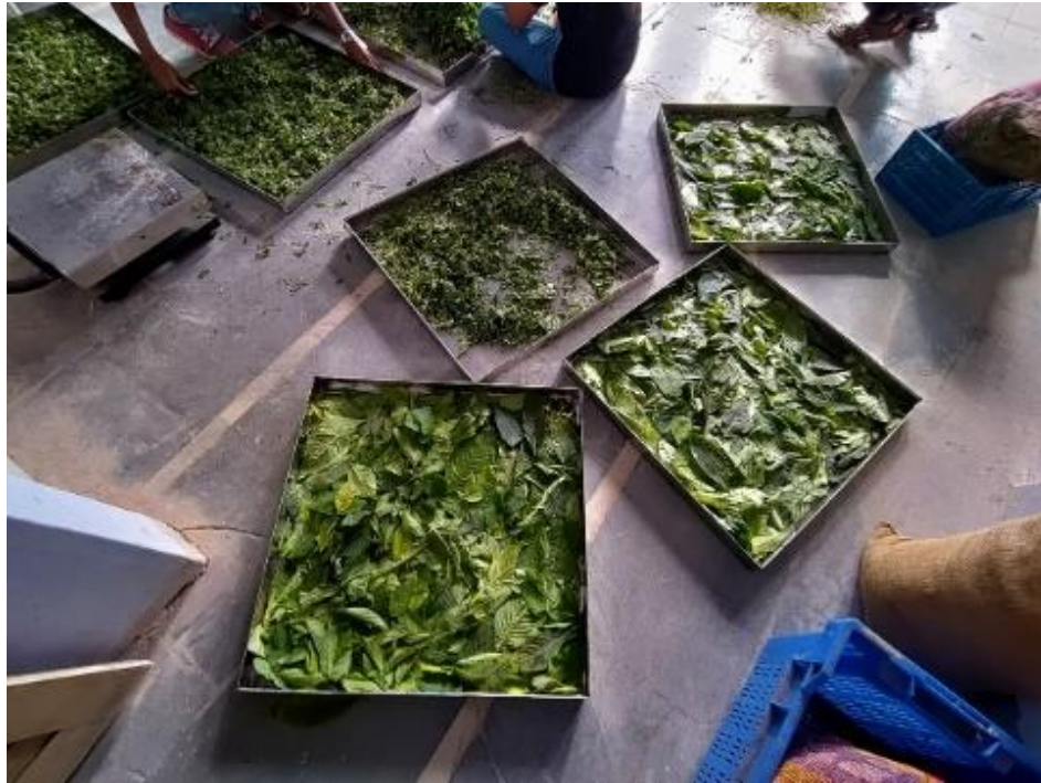
Plate 3.15 (a) Loading of samples in SS drying tray
