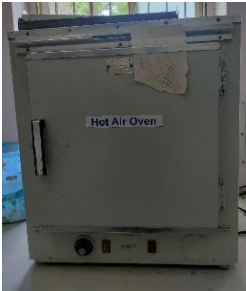
Plate 3.17 Hot air oven for determination of moisture content
