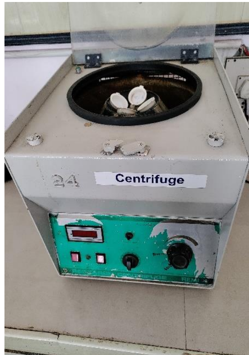
Plate 3.30 (a) Centrifuge machine for WAI determination
