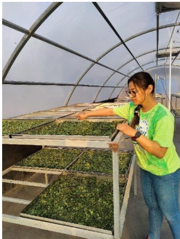
Plate 3.15 (b) Loading of SS trays in solar tunnel dryer
