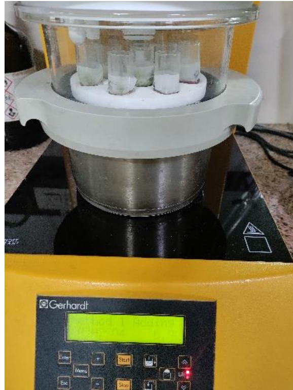
Plate 3.24 Fibre extraction process of the samples
