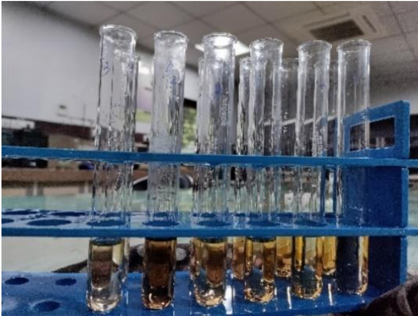
Plate 3.16 Carbohydrate extraction of the samples
