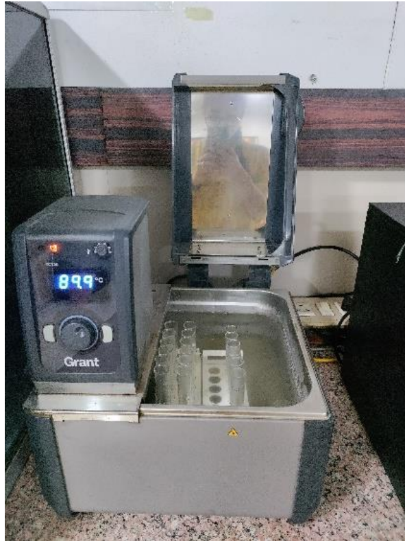
Plate 3.18 Water bath used for determination of ascorbic acid
