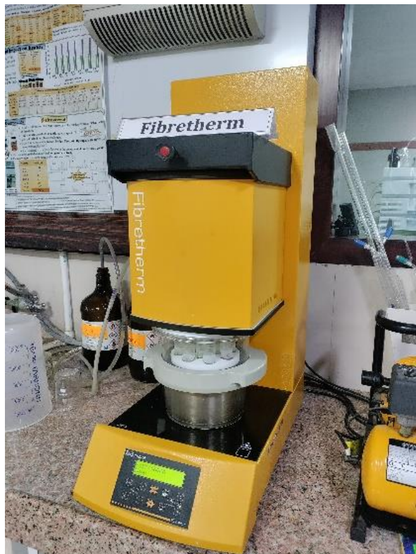
Plate 3.23 Fibretherm used for determination of fibre content
