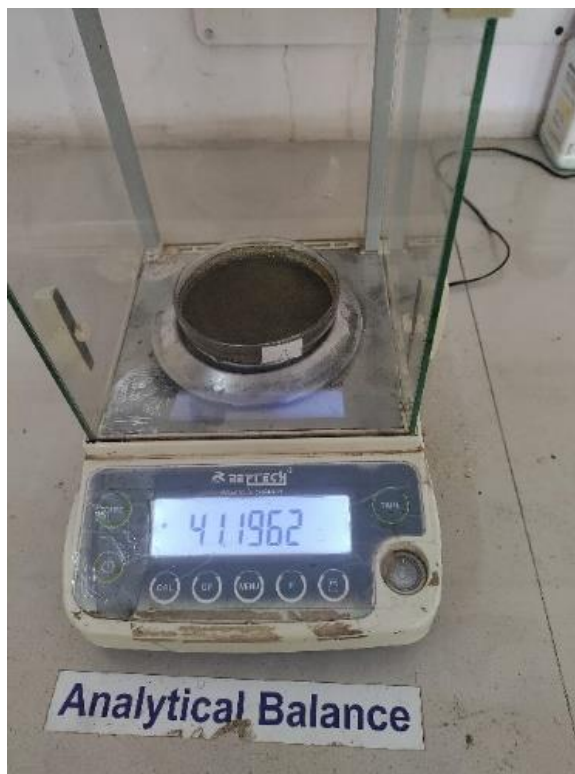
Plate 3.27 Analytical weighing balance used for physio-chemical analysis
