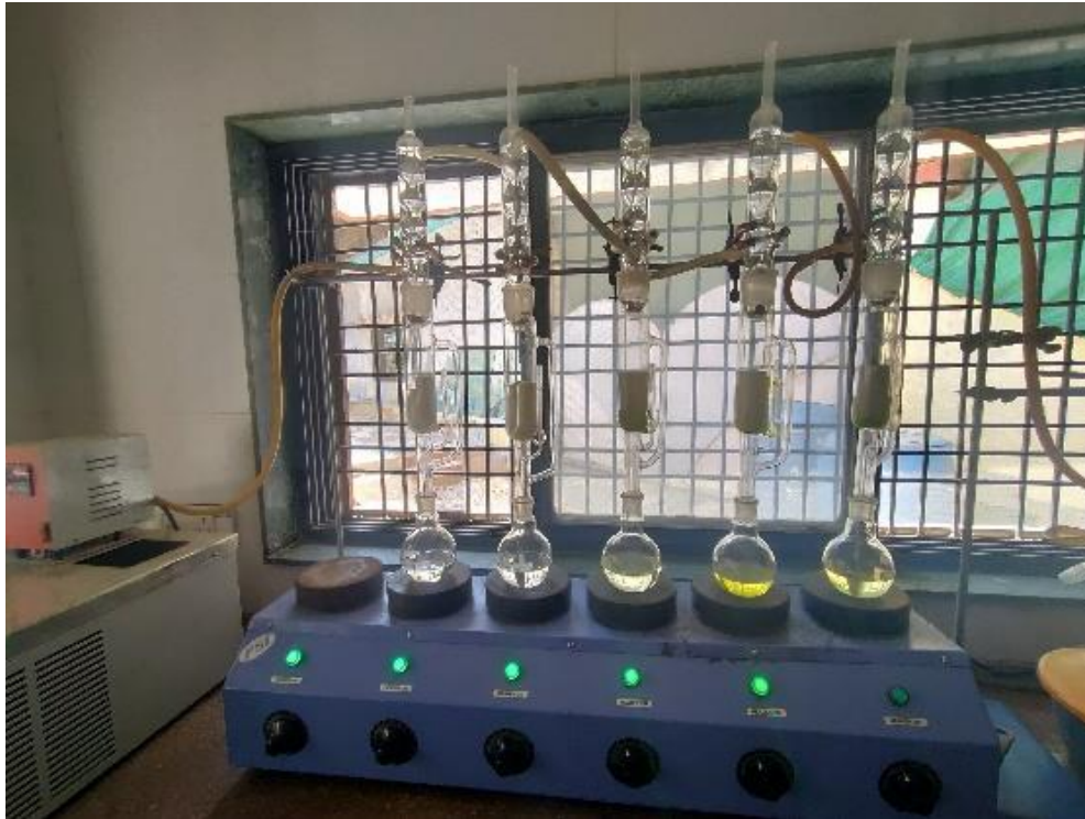
Plate 3.20 Soxlet apparatus for determination of fat content
