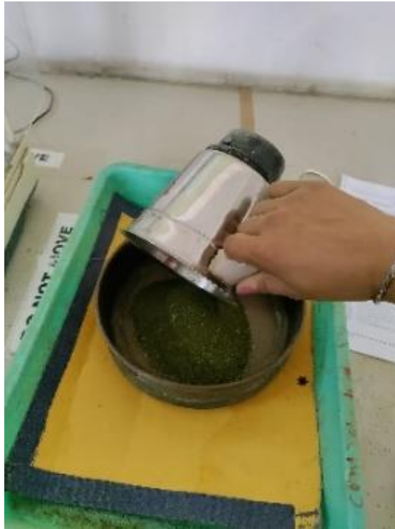
Plate 3.28 (c) Pouring of Adhatoda vasica leaf powder into the sieve (300 \mu )
