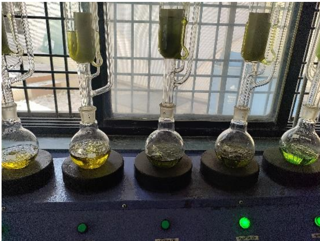
Plate 3.21 Fat extraction process for the samples
