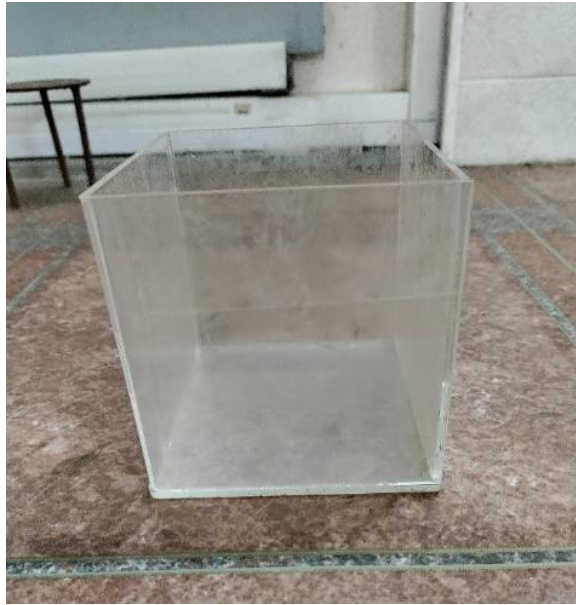
Plate 3.26 Container used for determination of bulk density
