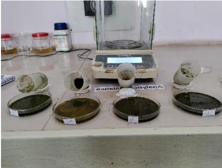
Plate 3.29 (a) Supernatant for WSI determination of the samples
