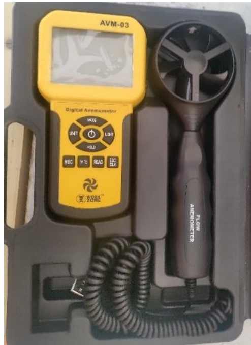
Plate 3.11 Anemometer for wind velocity measurement
