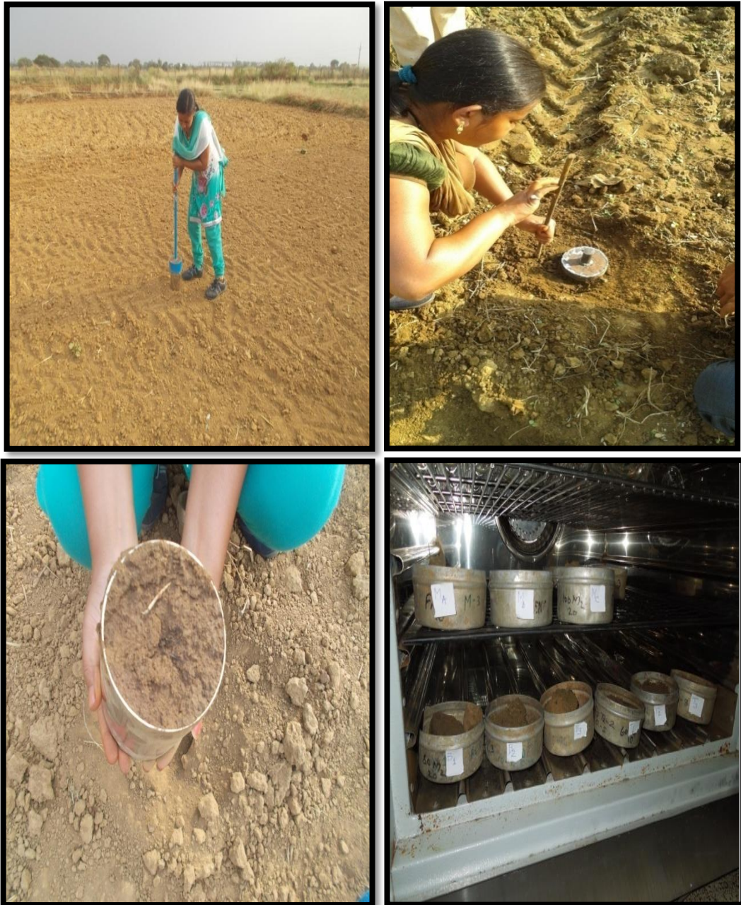
Plate No 3.7 : Find out moisture content using core cutter
