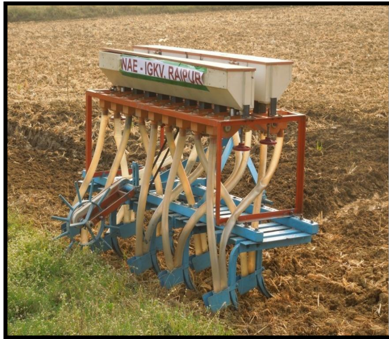
Plate 3.2 : Automatic seed cum fertilizer drill
