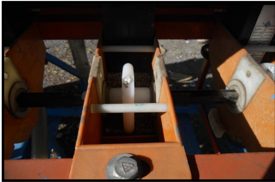
Plate 3.4 : Seed metering and dropping mechanism The metering rollers specification were given in Table 3.2
