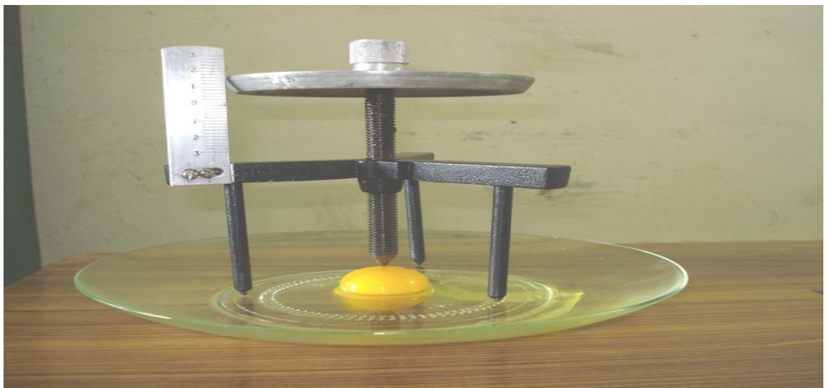
Fig. 8 Measurement of yolk height by spherometer
