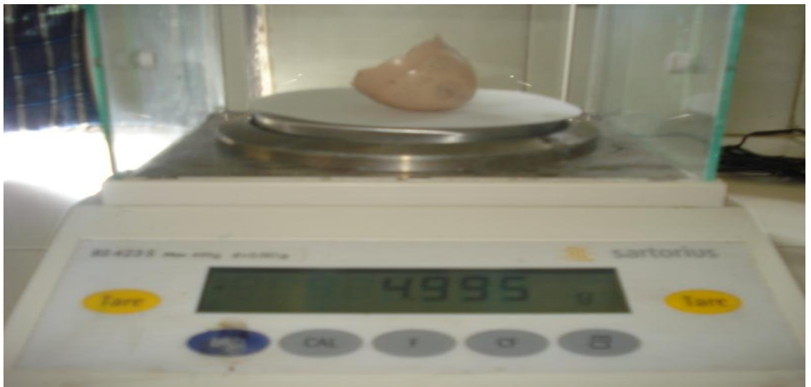
Fig. 14 Measuring of egg shell weight by electronic weighing balance
