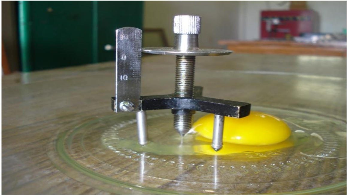
Fig. 13 Albumen height measuring by Spherometer
