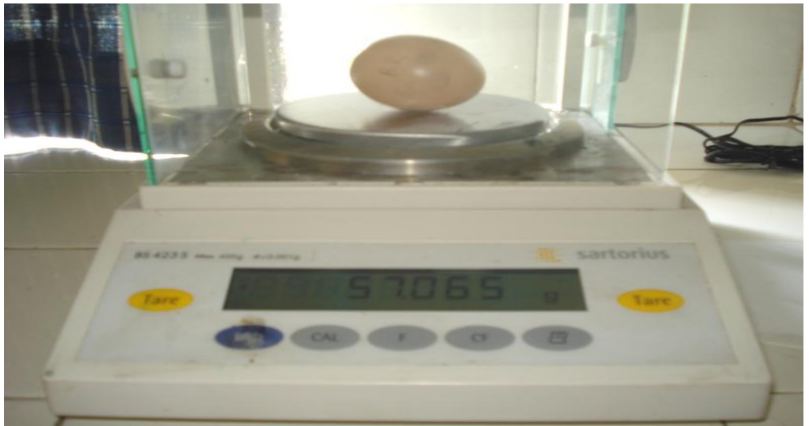
Fig. 15 Measuring of egg weight by electronic weighing balance
