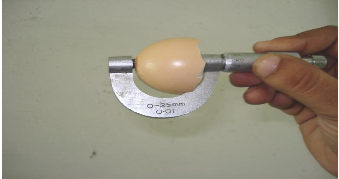
Fig.9 Measuring shell thickness by screw gauge
