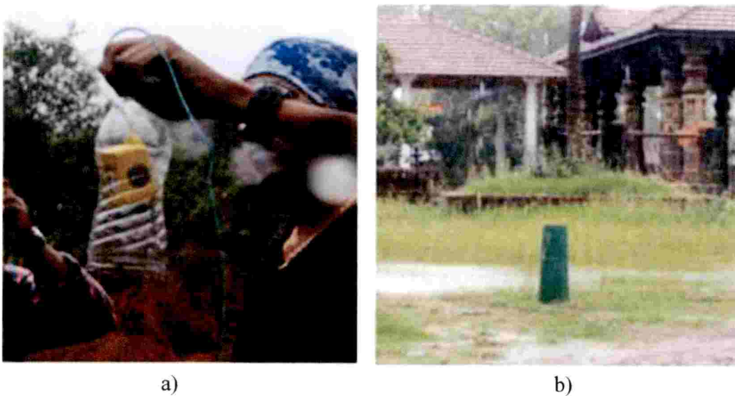
Figure 1. Instruments used for measuring weather parameters a) Temperature, Humidity sensor b) Rain gauge for measuring rain
