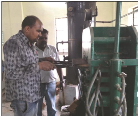
Plate 16: Preparation of particle board by using hydraulic hot press
