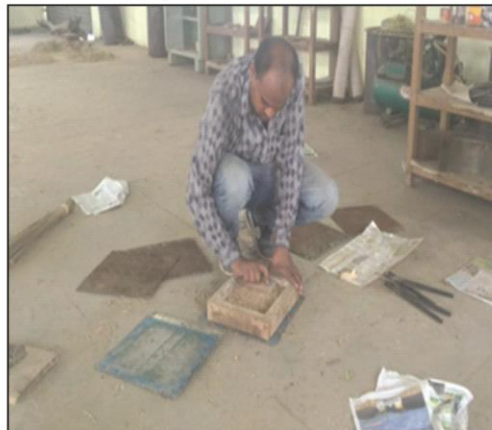
Plate 14 : Mat formation by wooden mould
