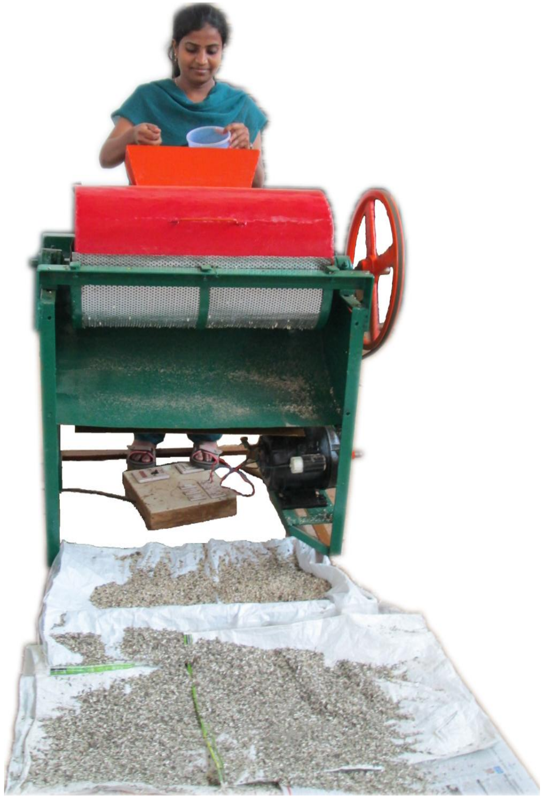
Plate 3.7 Power operated sunflower seed decorticator in operation
