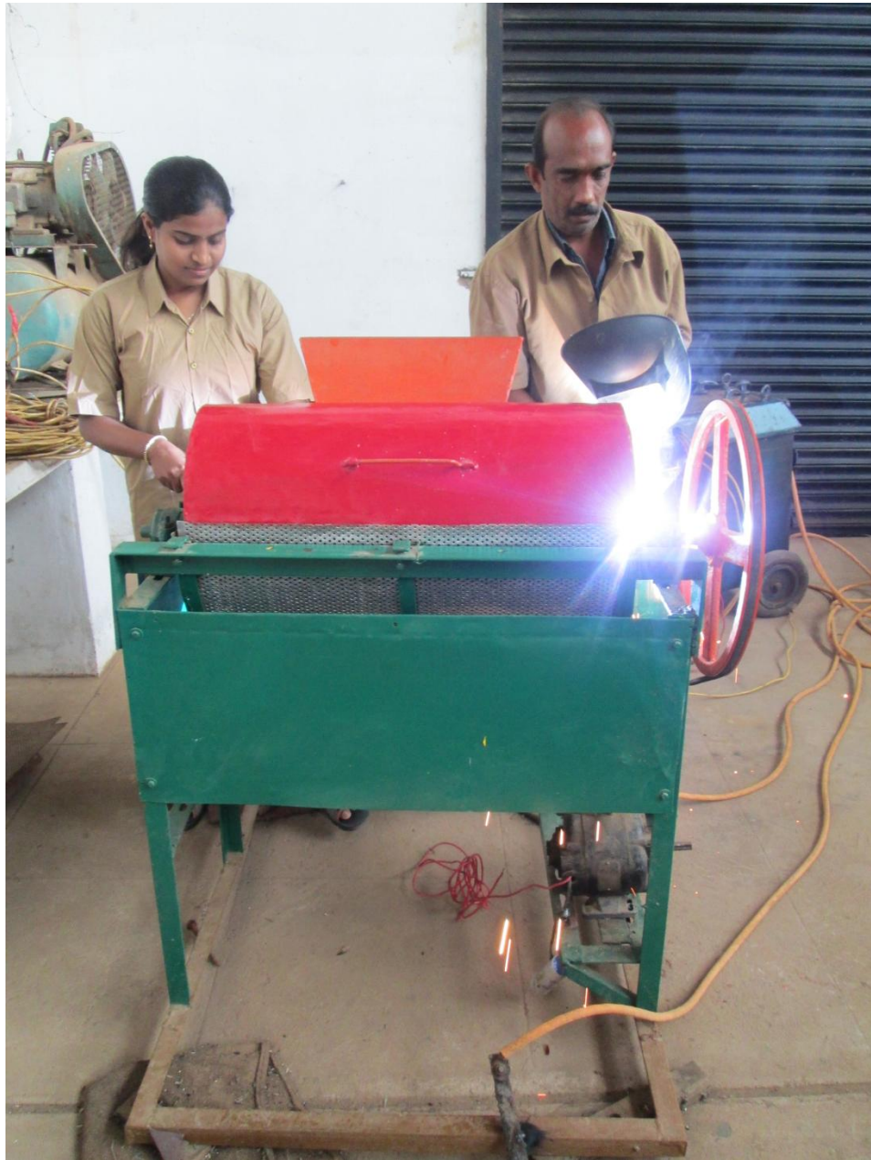
Plate 3.5 Fabrication of frame
