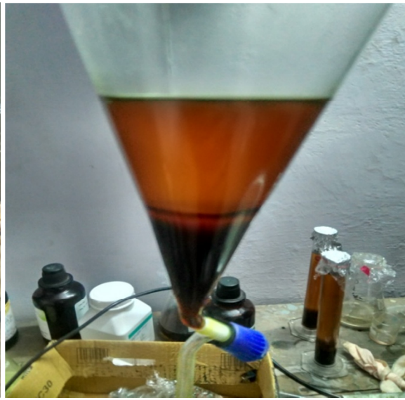
Fig. 3.4(b): Biodiesel floated up in separating funnel
