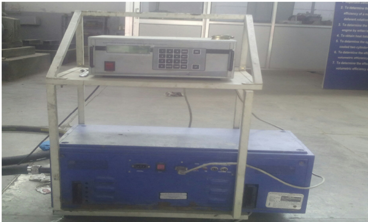
Fig. 3.14: Photographic view of Exhaust gas monitor
