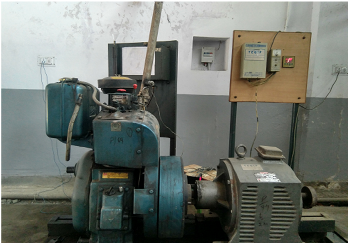
Fig. 3.13: Diesel engine with eddy current dynamometer
