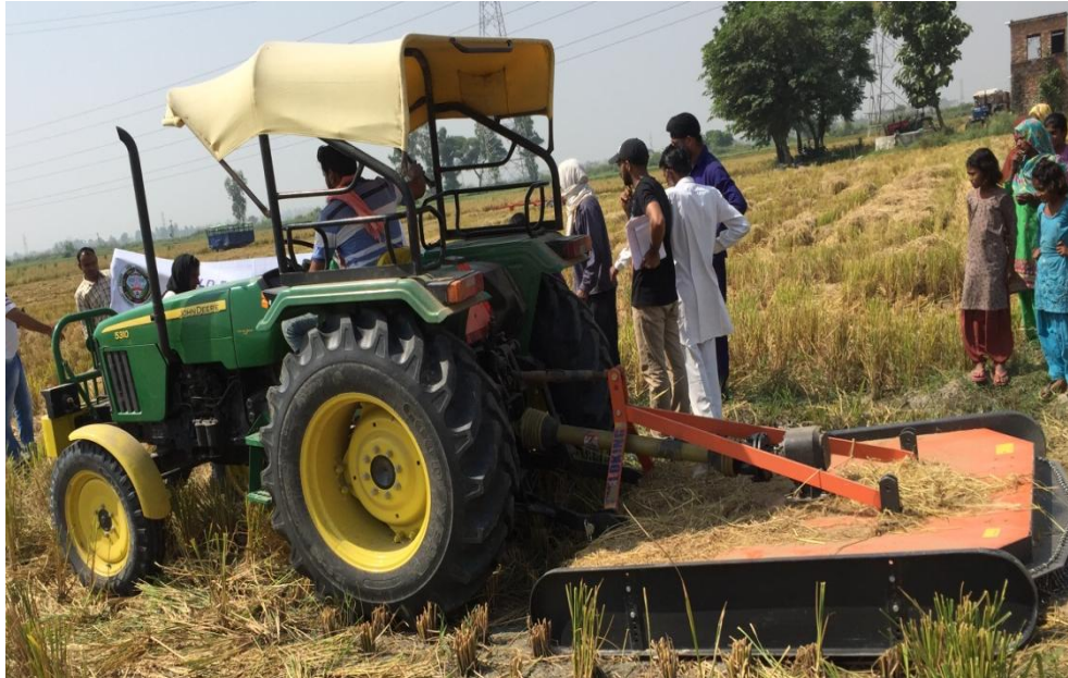
Plate 3.3 View of stubble shaver attached to PTO of tractor for operation in field
