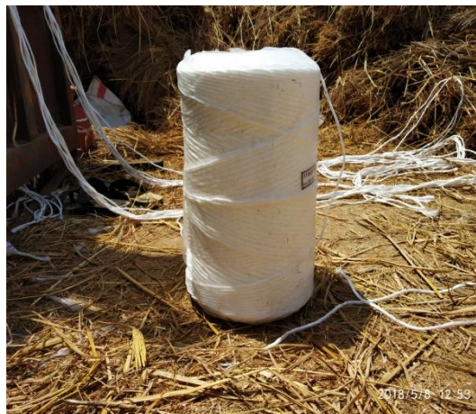
Plate 3.2 Poly propylene rope twine used for tying bale in stationary baler
