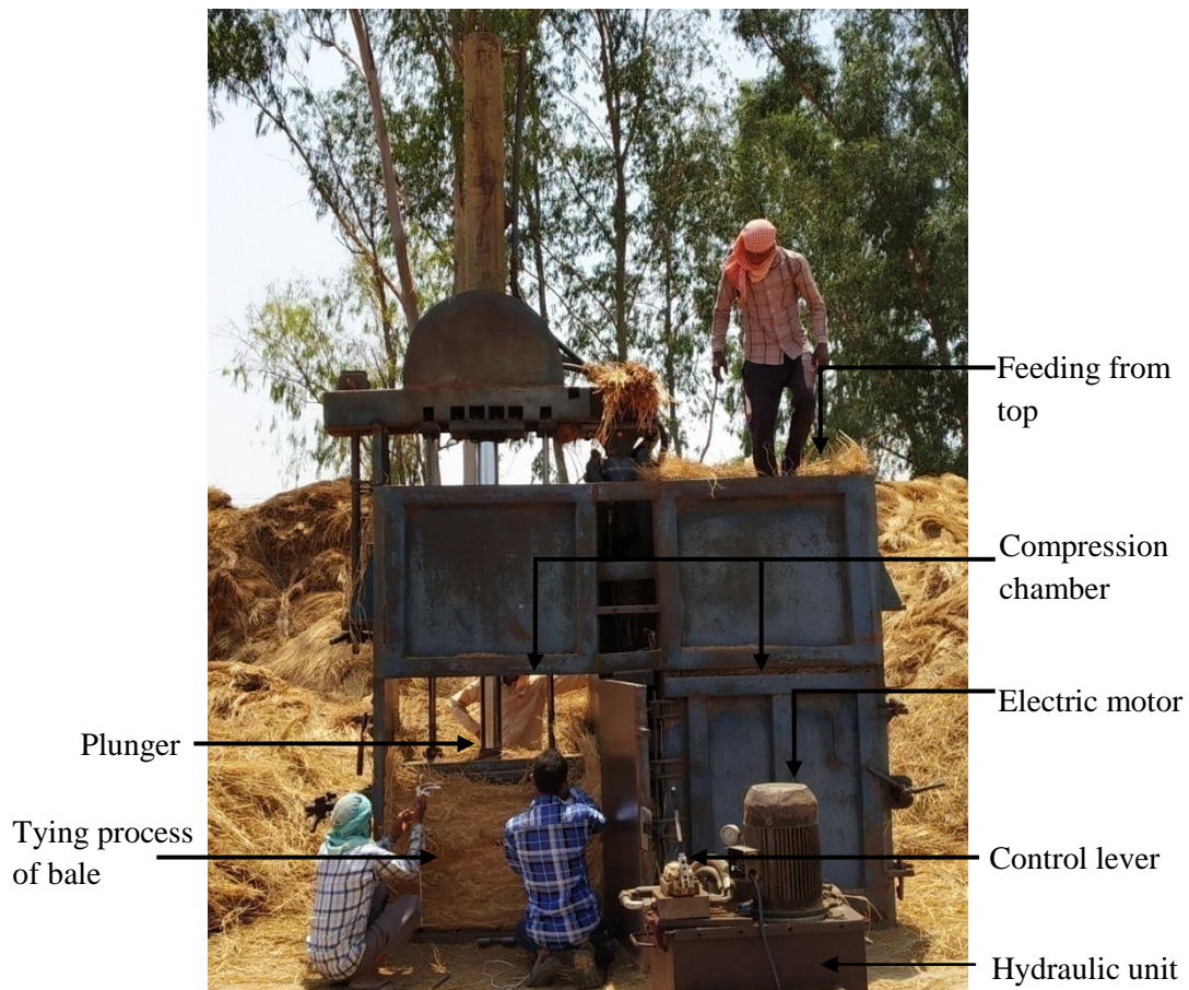
Plate 3.5 Front view of stationary baler for full length straw densification
