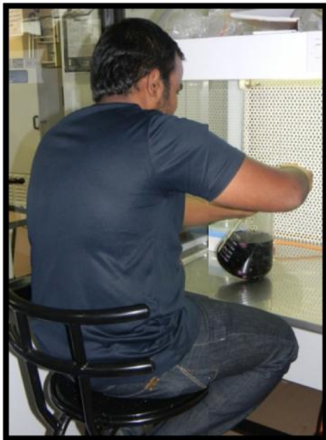
Addition of inoculum after cooling in sterilized condition
