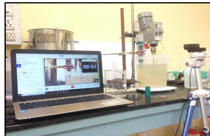
Fig. 3.4: Experimental setup of electrical conductivity method
