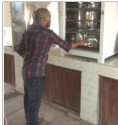
Determination of Dry Matter
