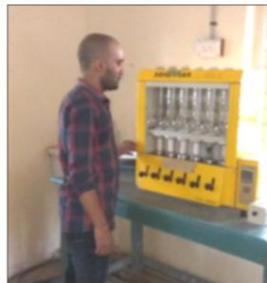
Determination of Ether Extract
