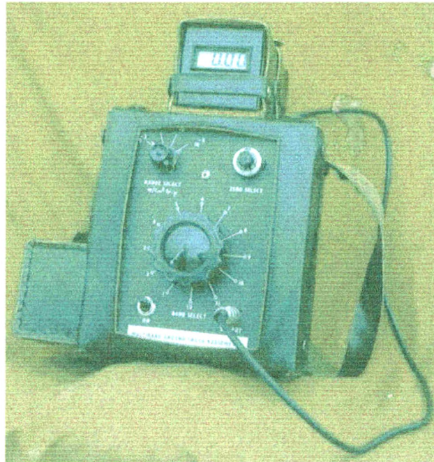
Plate 2. Opto -Mech Multiband Ground Truth Radiometer
