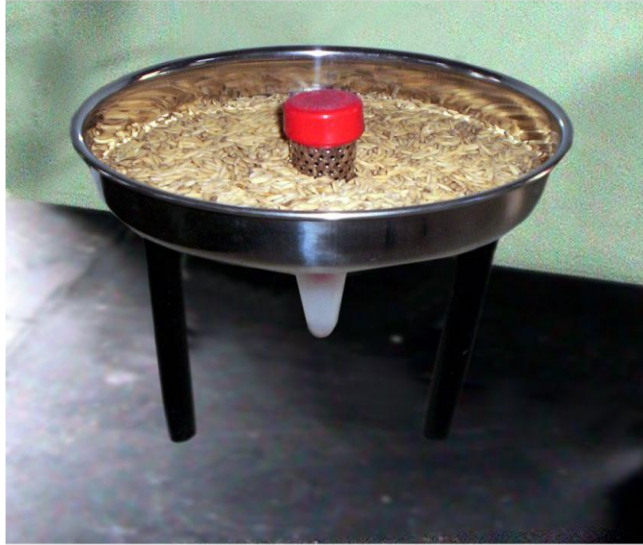
Plate 5. Three-in-One bioassay unit with test grains
