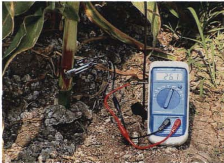
Figure 4: Analysis of root capacitance of genotypes using a Root Capacitance Meter
