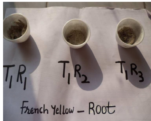
Plate-6 : Determination of carbon content (%) by Ash method
