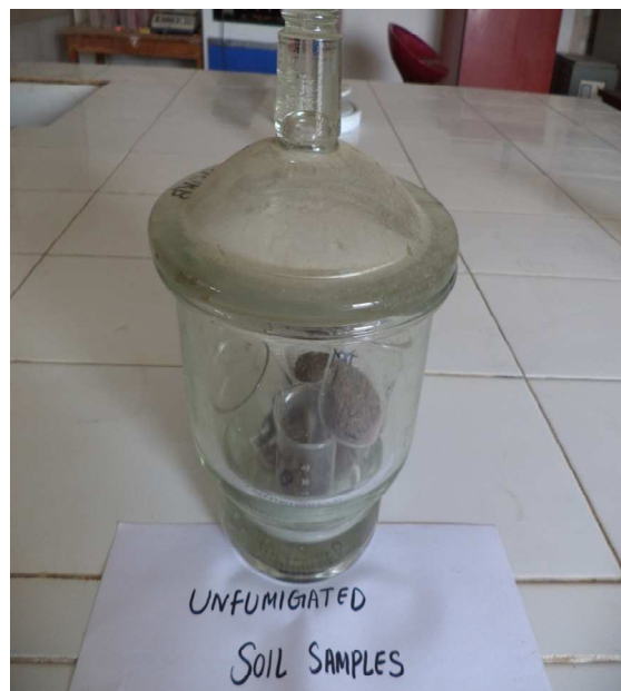
Plate-7 : Determination of soil microbial biomass carbon by chloroform fumigation extraction method
