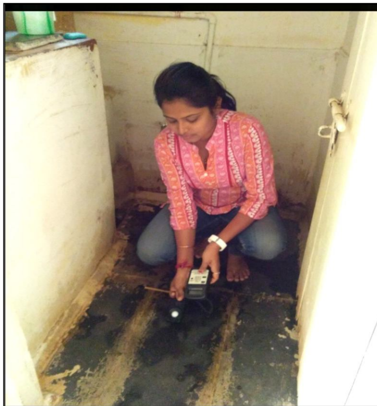
Plate 6: Measurement of light using lux meter
